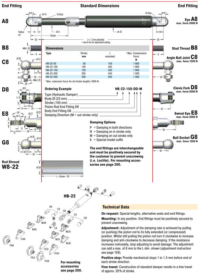
Material: Body: Black coated steel. Piston rod: With wear-resistant coating. End fittings: Zinc plated steel.
